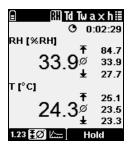
The **Statistics view** shows the current value of the selected parameter, as well as the maximum, average, and minimum value since the measurement was started. There is also a counter that shows how long the measurement has been running.
