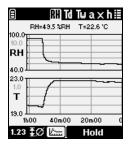
Switch to the Graph view and wait until the graphs level out, indicating that the measurement is now stable.
