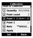
The correction to the measurement at point 1 is now shown in the text for menu item [3]. If you are only doing a 1-point calibration, skip to step 8.
