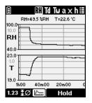
The **Graph view** shows a continuously updating graph of the selected parameter and temperature.
