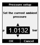
In the **Pressure setup** screen, you can set the current ambient pressure. The pressure information is used when calculating certain humidity parameters, such as mixing ratio (symbol x).
